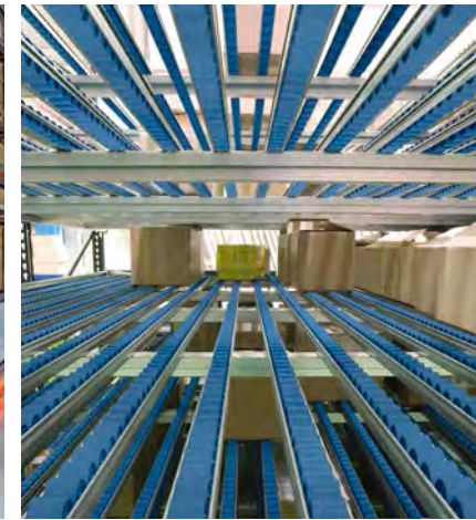
Carton Flow Racks - FIFO Wheel and roller platforms for visibility and faster configuration.
