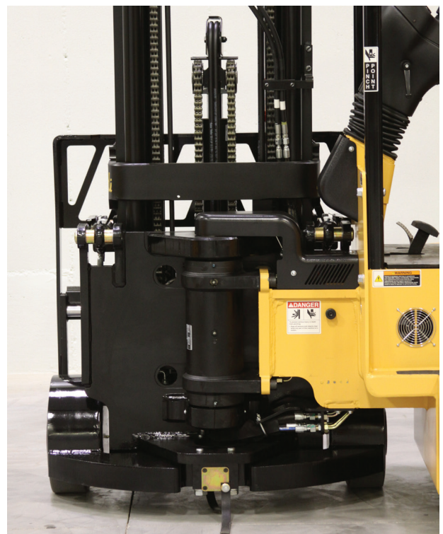
DuraSteer™ Front Wheel Steering *Patented
